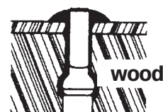
GROOVED RIVET Grooves improve holding strength
